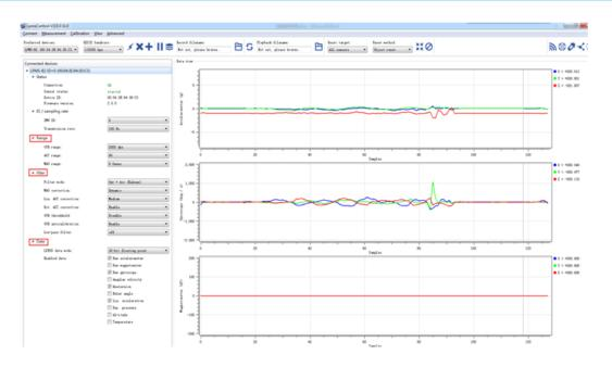
On the left side of the main interface of LpmsControl, users can change the sensor settings, like measurement range, filter modes, data updating rate, etc. Moreover, the types of output data can be modified by checking or unchecking the check box of each parameter. For example, in the following image the "raw magnetometer" is checked so that the acquisition of magnetic data is enabled.
