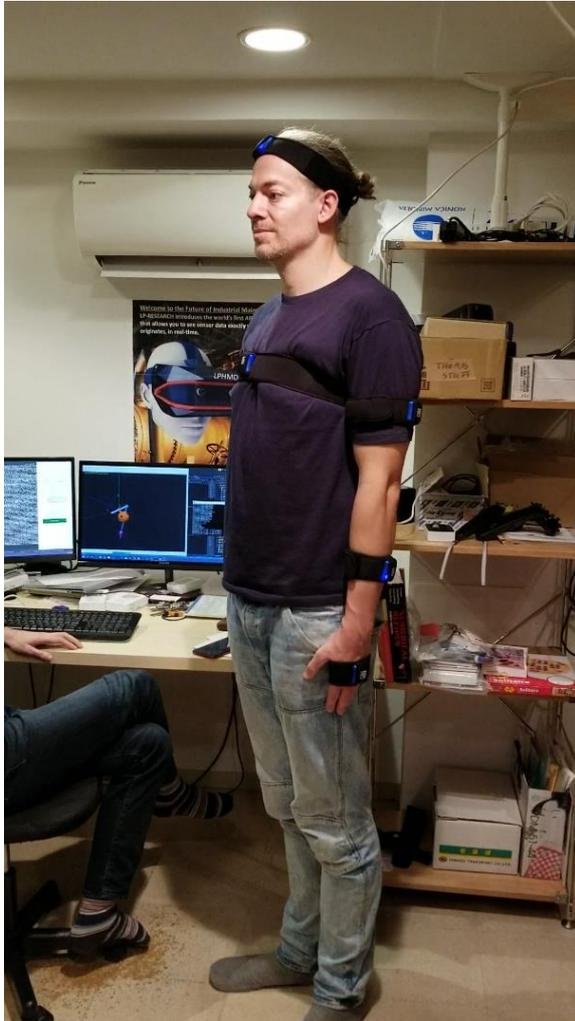
Figure 12 - Calibration neutral pose
