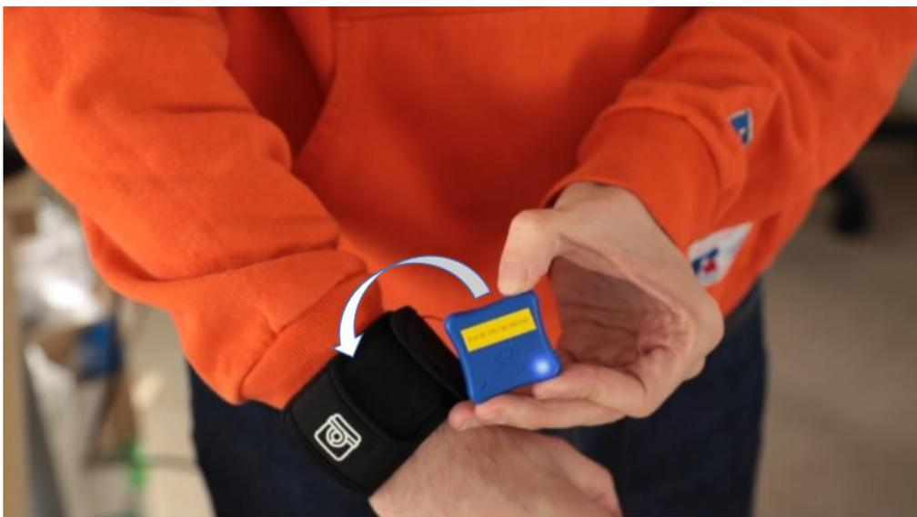
Figure 5 - LPMS-B2 is inserted into a holder strap that is attached to the user's body
