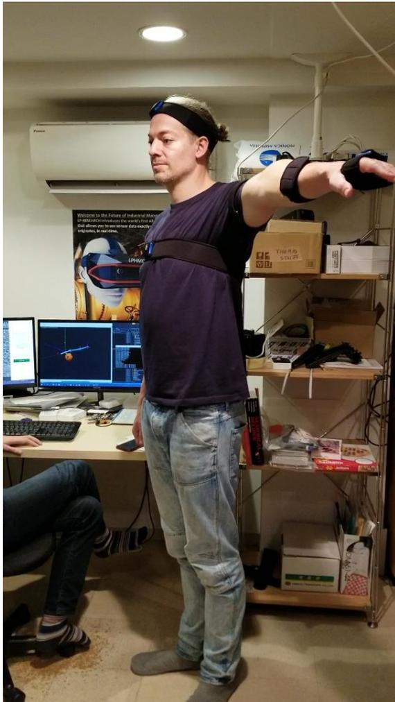
**Figure 10 - Calibration T-pose; the palms of the hands should be facing downwards (thumbs forward).**
