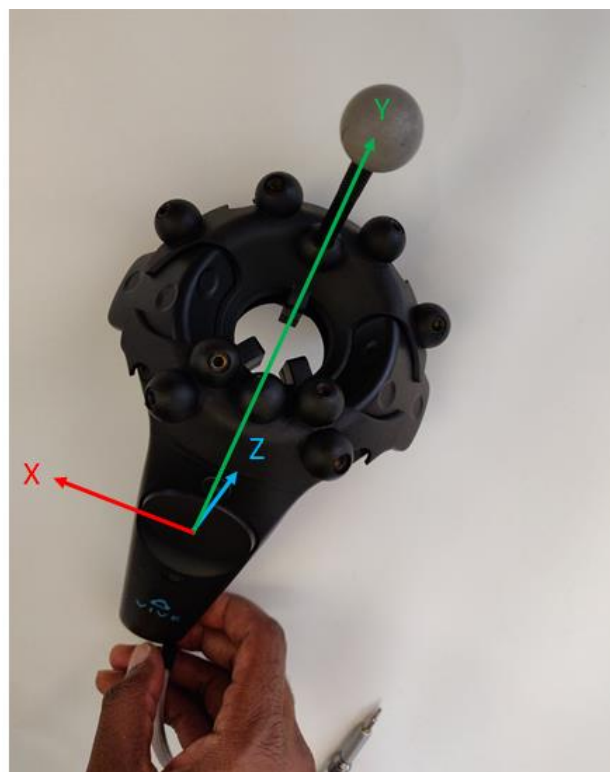
Figure 16 - Alignment of the controller coordinate system (defined in OpenVR): X-axis pointing left, Y pointing upwards along the handle and Z pointing perpendicular into the touchpad. Note that in this image just one marker post is attached, but at least 3 markers are required for proper optical tracking.
