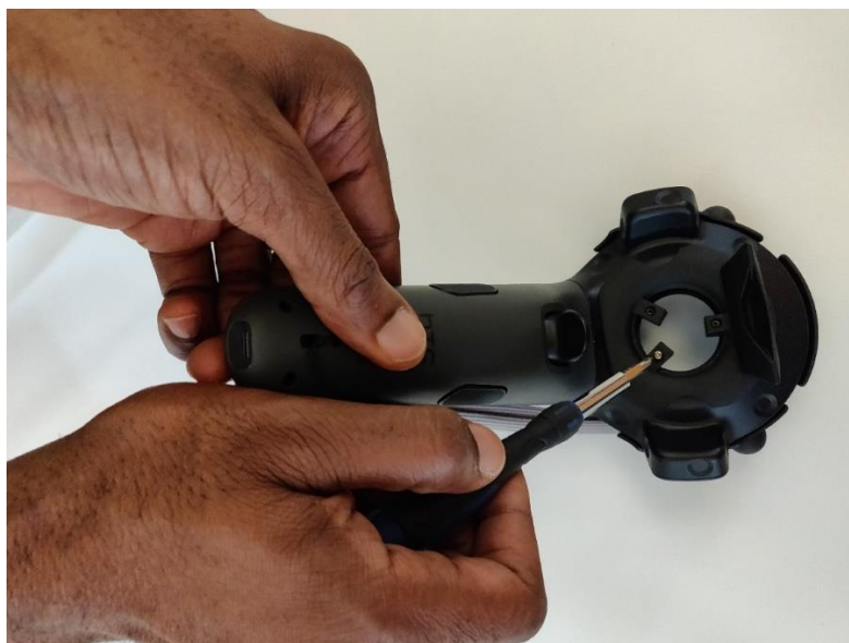
Figure 24 - Align the holder components with the hand controller as shown in the image and connect them using the screws delivered with the set.
