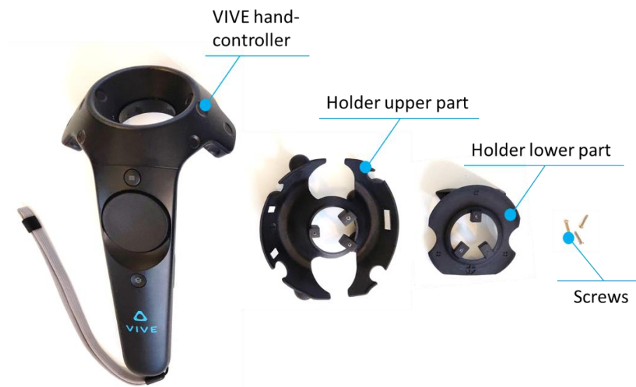
Figure 23 - The upper and lower part of the maker holder needs to be assembled around the VIVE / VIVE Pro hand controller.
