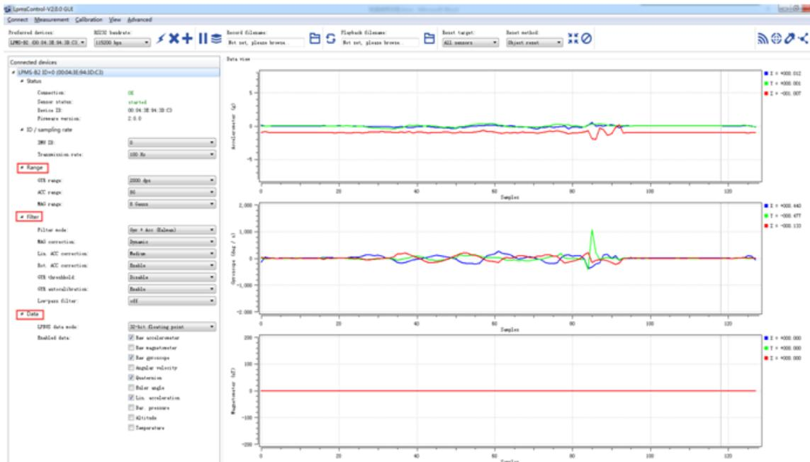
On the left side of the main interface of LpmsControl, users can change the sensor settings, like measurement range, filter modes, data updating rate, etc. Moreover, the types of output data can be modified by checking or unchecking the check box of each parameter. For example, in the following image the "raw magnetometer" is checked so that the acquisition of magnetic data is enabled.
