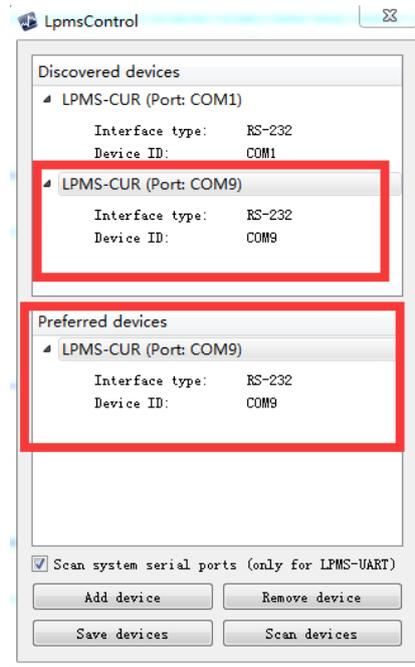
12) To select the target sensor ID from the Preferred devices list, and click Connect function under "Connect" menu or click the lightning button on toolbar to connect the sensor. Note: The default baudrate of UART communication is 115200bps.
