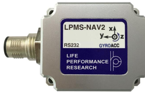
Fig. 3.1. Sensor coordinate for TTL/RS232/RS485/RS422 models
